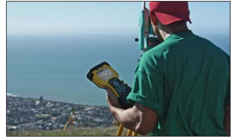
Connect a TDS Ranger for more data collection capabilities You can expand your data collection capabilities by connecting a TDS Recon or Ranger (shown) data collector to the 302 Series total station.
